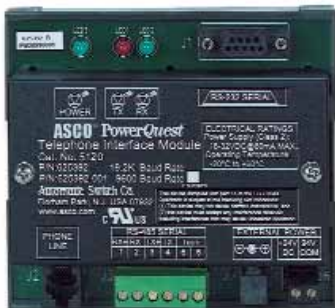
Fig. 13: Telephone Interface Module
